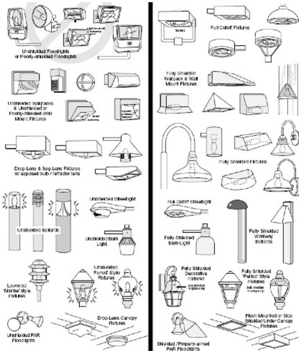
Figure D: The lights on the left are non-conforming. Those on the right may be used in most cases. However, the mounting height and proximity to the property line may require additional shielding to prevent the luminous elements from being visible from any other property.
